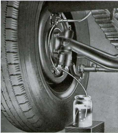
Fig. 35 Bleeding front wheel cylinders.
