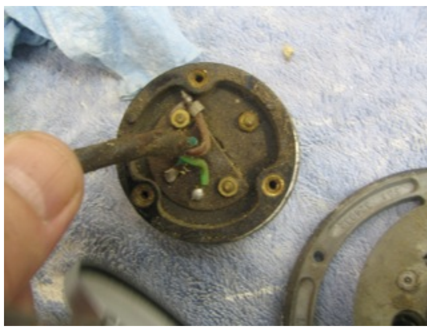
Once the three screws are removed, the switch will separate into two halves, one that will be attached to the horn ring and one that connects to the stator tube. Pull them apart including pulling the long wire harness up and out of the tube.
