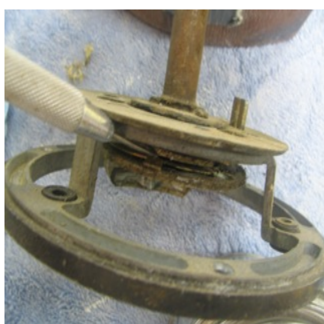
Thin brass cover plate that has to be rotated to expose the three screws that hold the assembly together
