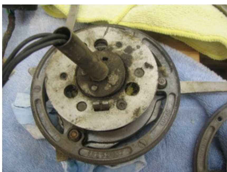
The back of the turn signal assembly with the long stator tube removed. Note the three holes to access the screws that hold the assembly together.
