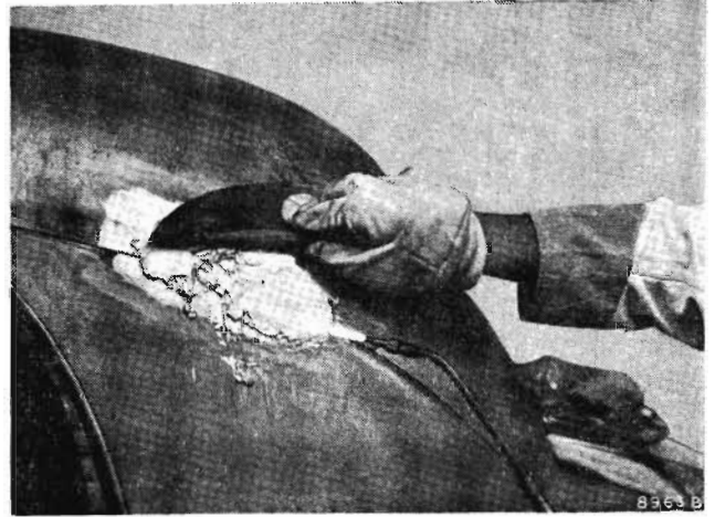
Fig. R.21 Spreading the solder
